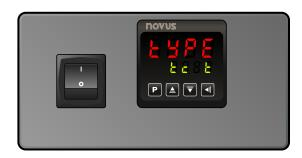
Press and release the **P** button to toggle through the menu until you see "unit" displayed in red. The green text will read **°F** for Fahrenheit or **°C** for Celsius. Press the up or down arrow buttons to change to your desired unit. Once changed press and release **P** to continue through the menu.
