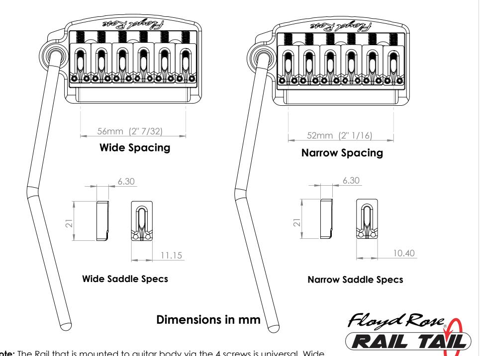
**Note:** The Rail that is mounted to guitar body via the 4 screws is universal. Wide and narrow spaced tremolo plates are interchangeable with any Rail.
