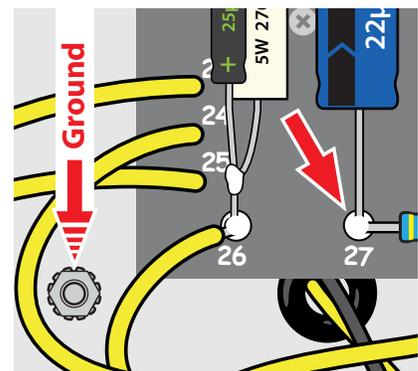
Set your multimeter to 500V DC and connect the black (negative) probe to ground. Once that probe is secured to ground, measure the DC voltage at eyelet 27. This B+ voltage should be roughly 510V DC.
