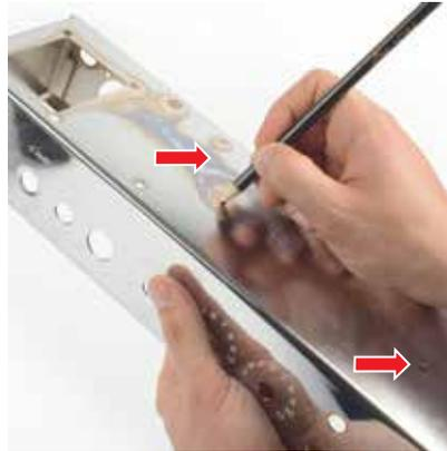
Holding the boards in place, turn the chassis so you can see the two mounting holes. Using a sharp pencil through the holes, mark the hole locations onto the insulator board.
