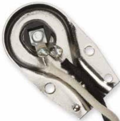
Trim the black lead to fit and solder it to the sleeve lug. The solder joints need to be neat in this metal case. Reassemble the plug.
