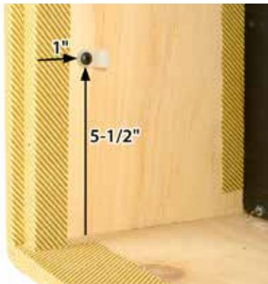
Don't drill through the cabinet! Use a piece of masking tape on your drill bit to mark the depth, or use a StewMac Depth-stop Drill Bit (item #1712).
