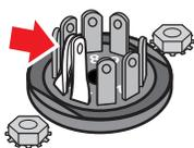
On the V2 socket and the V1 socket, twist pins 4 and 5 toward each other so that their eyelets line up.
