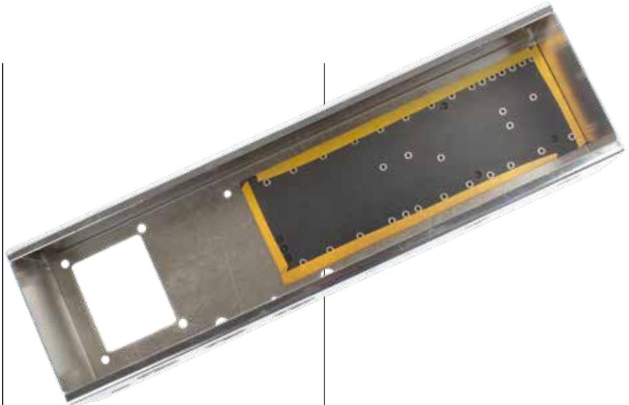
Position the taped boards inside the chassis as shown above, with a gap of roughly 1/4" between the long edges of the boards and chassis. The short ends of the boards are flush against the end of the chassis.
