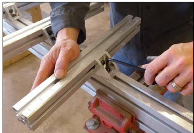
**1.** Install an angle support in each of the three crossbars. The T-shaped sliders fit the crossbars, and the square nuts are for mounting to the main beam. Two of the crossbars have etched centering scales, which should face upward.
