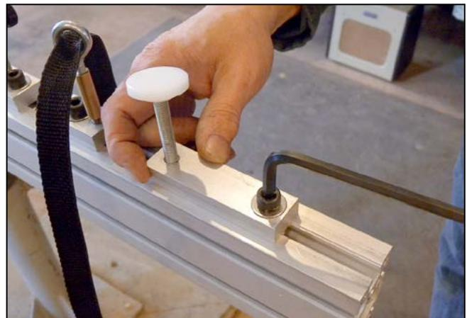
**8.** Install the peghead jack. The threaded leveler can swing to either side to support asymmetrical pegheads.
