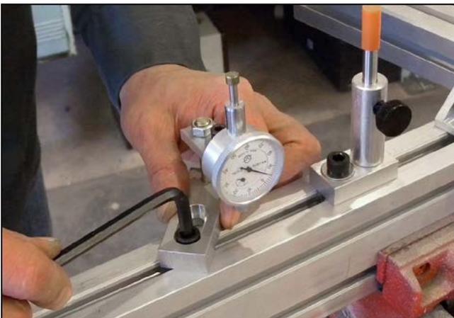
**5.** Attach the first dial indicator to the main beam. The dial's mounting bracket is offset, allowing the height-adjustable rod to move in relation to the main beam.
