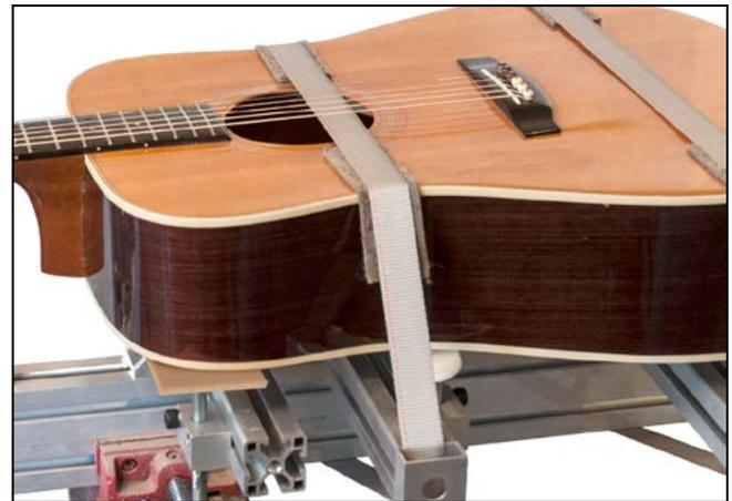
**Warning about acoustic guitars:** Before jiggging an acoustic, think about the guitar body's internal construction. The body must be supported under the strong kerfed joint where the back meets the sides, not at the unsupported areas of the back.
