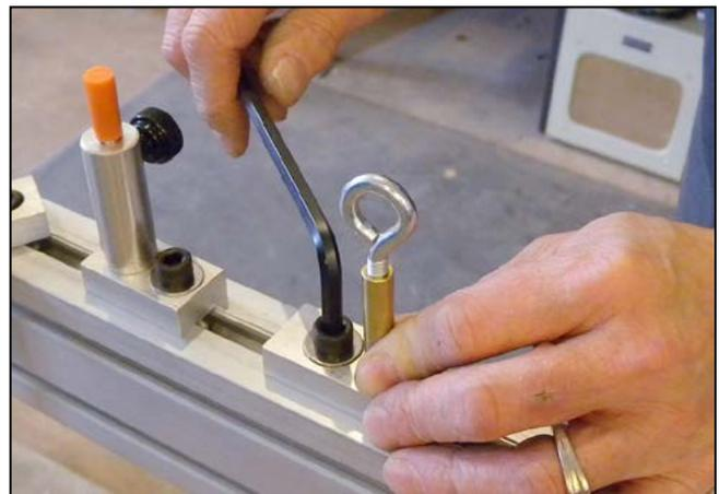
**7.** Attach the peghead puller and thread the strap through the eyebolt.
