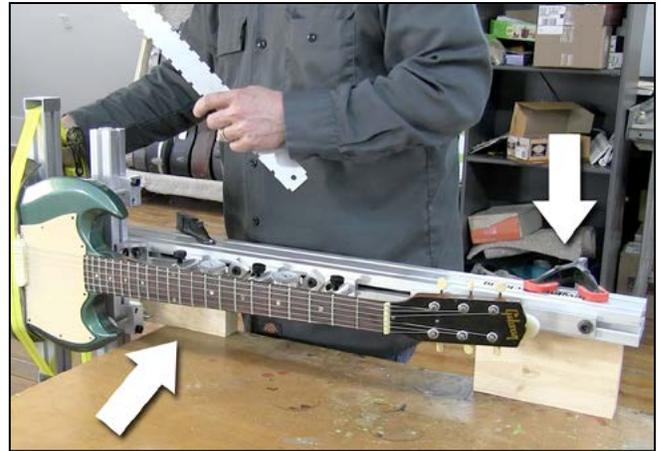
To rotate the Neck Jig into the playing position on a benchtop, place two wooden blocks under the main beam. Use two bar clamps to hold the Jig and blocks to the bench. The guitar body is suspended off the end of the bench.
