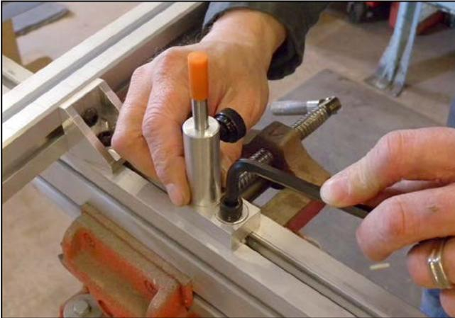
**3.** Install a neck support rod on the main beam. These three rods adjust vertically to support the instrument neck. The bottom end of the rods drop down into the slot in the main beam.
