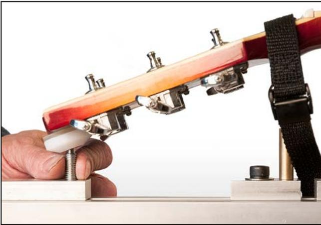
**10.** Slowly raise the peghead jack until the dials read zero again. If the rear dial is off, tighten down the peghead strap until zeroed. Go back and forth between these adjustments, until both dials remain as close to zero as possible.
