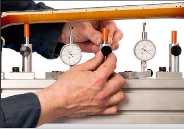
**⚠ Caution:** Before tightening the body straps, lower the neck support rods. Tighten the hold-down strap gradually until the guitar body is snug on the levelers. Sometimes a guitar will require two straps in order to secure it on the levelers.
