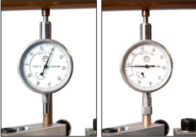
**9.** The neck will backbow with the strings removed, and the dial settings will no longer read zero. In our case, the dial nearest the nut has compressed .031" (left photo) and the dial nearest the body has compressed .008" (right photo). These are typical readings.
