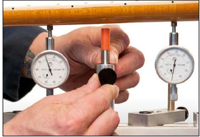
**11.** When the neck is re-zeroed to your satisfaction, slide the neck supports up against the back of the neck. These rods keep the neck from flexing while you level the frets or the fretboard.
