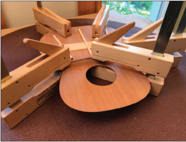
Optional: showing the gluing setup with clamps.
