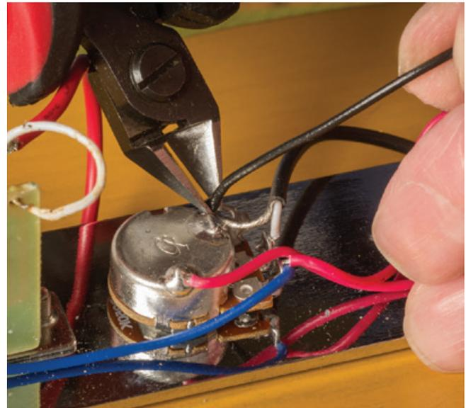
Note that there is one lead that is not necessary for this circuit. Cut this wire off at the volume pot.
