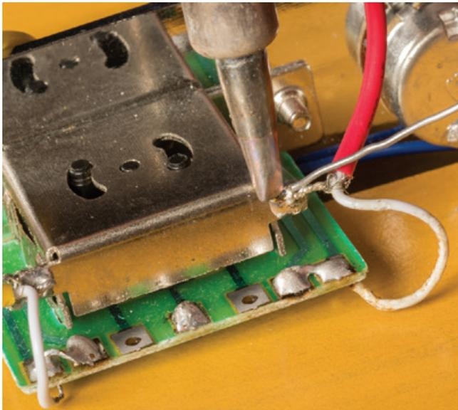
Solder the bare ground leads of each pickup to the lugs on the switch housing.
