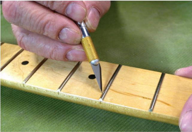
After the finish has cured, it's time to level and dress the frets. If you have a maple fretboard, lightly score the lacquer along the length of the frets with a sharp knife, using care not to cut into the wood or scratch the frets. This step helps in removing the lacquer that was sprayed over the frets during finishing.
