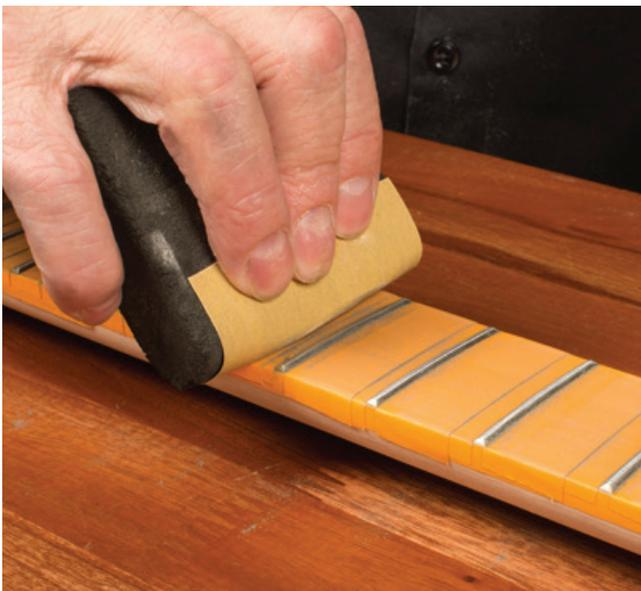
**Sand the frets** with 400-grit, then 600-grit sandpaper wrapped around a foam block, running up and down the entire length of the fretboard.
