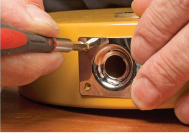
Mark the mounting holes for your jack plate, then drill pilot holes for the screws using a 1/16" drill bit.
