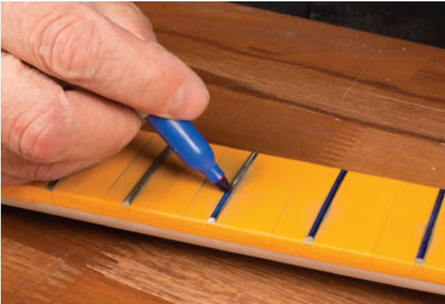
Color the fret tops with a blue permanent marker to prepare them for leveling. The blue ink will show your progress: the frets are level when sanding has removed some of the blue across all of the fret tops.
