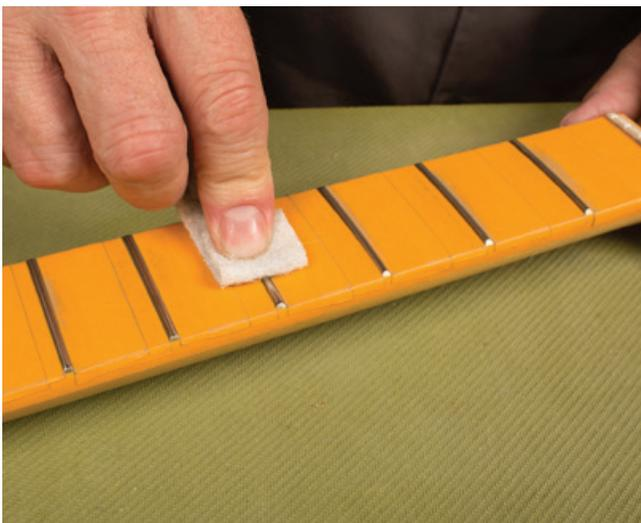
Follow up with Light Duty Scotch-Brite Pads or 0000 steel wool for a final finish. This will remove any of the remaining lacquer from the frets, and polish them to a smooth finish.
