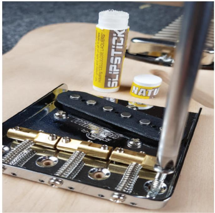
Drill the 4 bridge mounting holes deeper to accommodate the screws using a 1/8" drill. Mark the depth of the screw with tape on the drill after comparing the screw length. Countersink the hole slightly to avoid tearout when fitting the screws. Mount the pickup in the bridge and attach the assembly to the guitar. Lubricating the screw with a small amount of Slipstick will make the assembly easier
