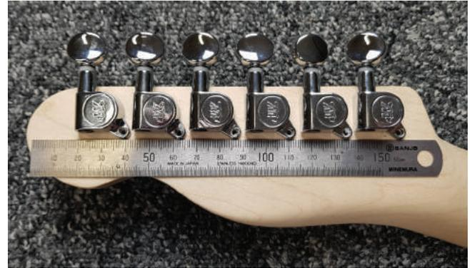
Lay out the tuners, using a ruler to make sure they're in line with one another and square to the edge of the peghead.
