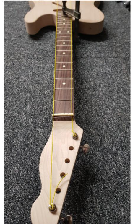
To align the neck and body I like to use a length of string/twine or thin hook up wire threaded through the E string ferrule holes in the body and then run the wire/ string up the neck through the nut to the E tuners to check alignment and make side-to-side adjustments to the neck as needed to make sure the strings ride even along both edges of the fretboard.
