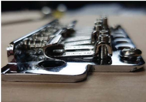
Attach the Wilkinson WVC vibrato using the 6 round head screws provided. (lubricate the screw threads with the Wilkinson "Slipstick" prior to inserting).
