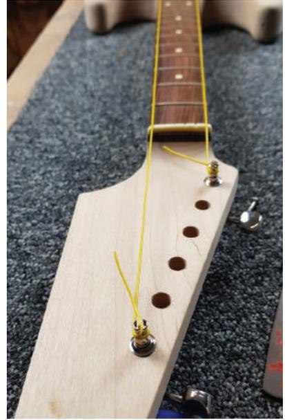
To align the neck and body I like to use a length of string/twine or thin hook up wire threaded through the E string holes in the block and then run the wire/ string up the neck through the nut to the E tuners to check alignment and make side-to-side adjustments to the neck as needed to make sure the strings ride even along both edges of the fretboard.
