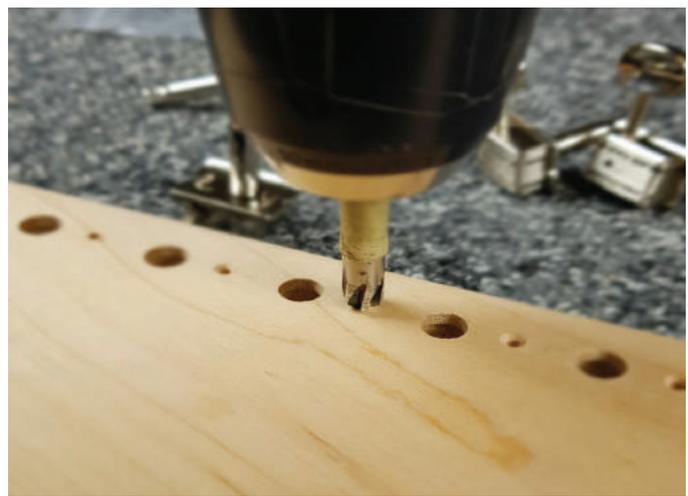
Mark out your mounting holes with a scribe or punch. Tuner mounting screws are very delicate and will break off if forced into hard maple. Use a 5/64" drill bit to make pilot holes for the screws; if these holes are any smaller you risk shearing off the screw heads.
