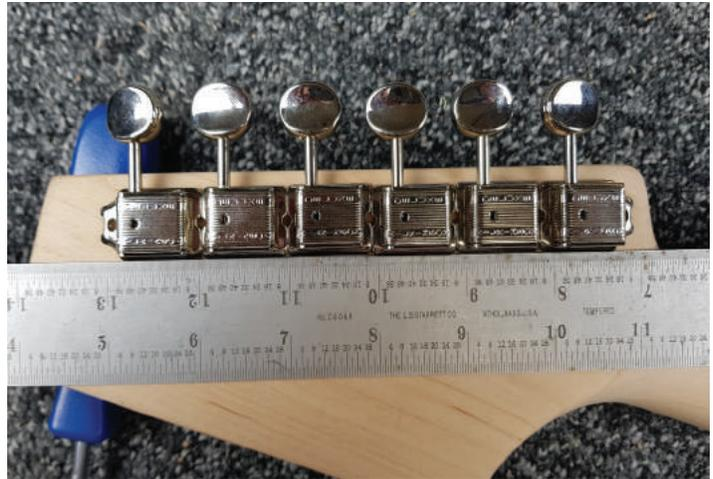
Lay out the tuners using a ruler to make sure they're in line with one another and square to the edge of the peghead.
