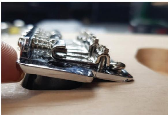
Install one spring in the centre of the spring block with enough tension on the claw to hold the bridge in place. I like to use the vibrato cover backing plate as a shim between the underside of the back of the bridge and the body, this not only stops the plate from damaging the body but later it will allow easy adjustment of the spring tension to give just the right amount of clearance allowing the bridge the clearance it needs to be a true floating vibrato.
