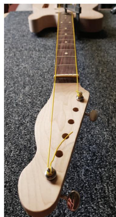
To align the neck and body I like to use a length of string/twine or thin hook up wire threaded through the E string ferrule holes in the body and then run the wire/ string up the neck through the nut to the E tuners to check alignment and make side-to-side adjustments to the neck as needed to make sure the strings ride even along both edges of the fretboard.
